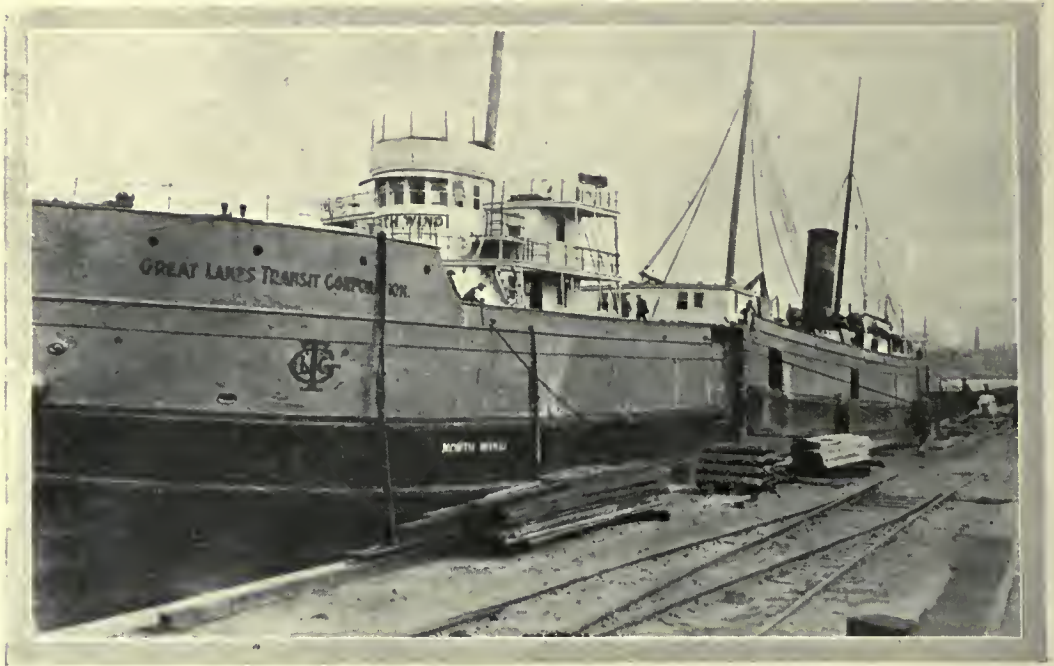
A LAKE STEAMER CUT IN TWO TO FACILITATE ITS TRANSFER TO THE ATLANTIC.
